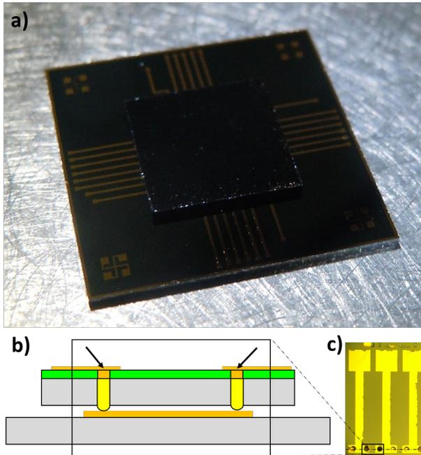
Figure 11: Electrical interconnect measurement procedure: (a) sample before backside removal, (b) schematic cross section view of a measurement of a single pair of bonded TSVs, and (c) top view microscope view.
