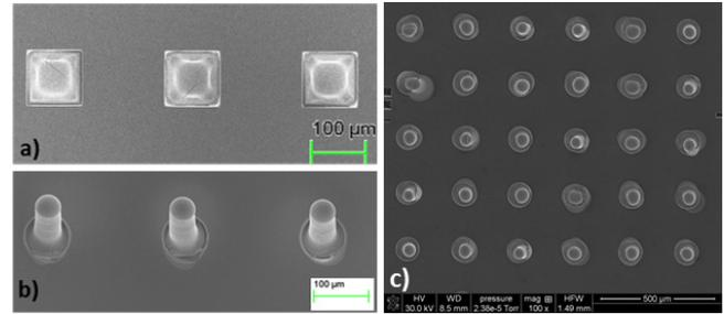
Figure 5: SEM micrographs of a) a linear array of 3 squares (80µm square length), b) 3 circular vias (40µm radius) and c) large arrays (partial view of 12x12 array).
