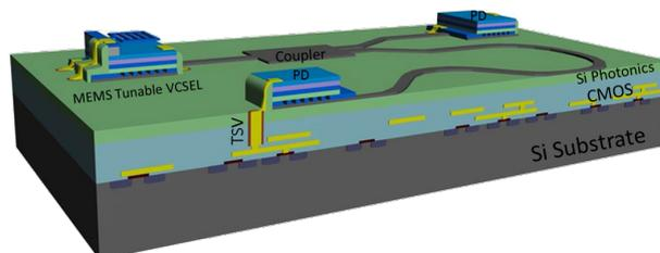
Figure 1: Heterogeneous integration of CMOS, Silicon Photonics and III-V active MEMS photonics in a single chip [1].
