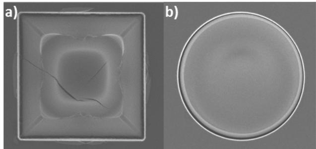
Figure 4: SEM top view images of single a) square (80µm square length) and b) circular  $r=40\mu\text{m}$  via filled with gold by inkjet printing (after sintering). The number of printed droplets was adjusted to completely fill the circular via.
