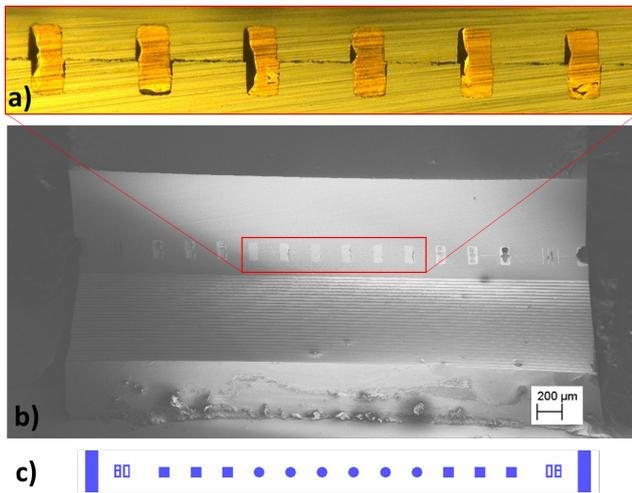
Figure 7: Cross section images of two bonded dies: b) SEM overview image and a) close up optical micrograph showing the 6 circular vias in the center, and c) the TSV etch pattern top view. The cross sections show good filling and repeatability of the process. Via radii are  $40\mu\text{m}$ .
