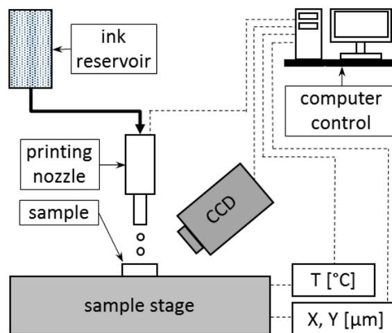
Figure 2: Inkjet printing setup at UC Berkeley [12].
