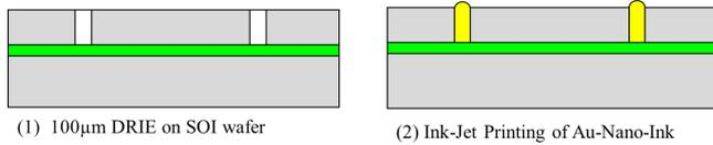
Figure 3: Schematic cross section representation of the ink-jet printed TSV sample preparation.
