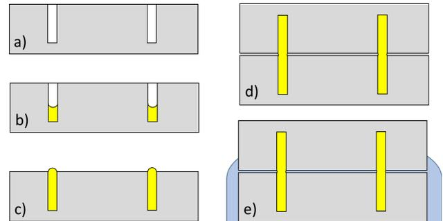
Figure 6: Schematic process sequence for TSV cross section visualization: a) wafer level DRIE of deep trenches, dicing; b) die level TSV filling and c) bond bump deposition in the same inkjet printing step. d) Die level alignment and bonding, including metal sintering and e) underfill for mechanical stabilization during cross section dicing process.
