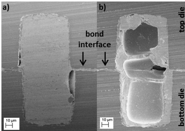
Figure 8: Cross-section images of diced Through Silicon Vias. The images reveal complete filling of the a) circular vias, while the (b) square vias are only covering the surface.
