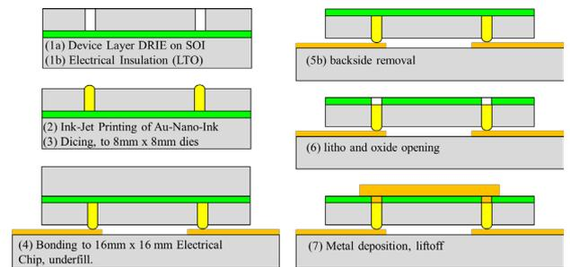
Figure 9: Sample preparation for bond strength and electrical interconnect measurements.
