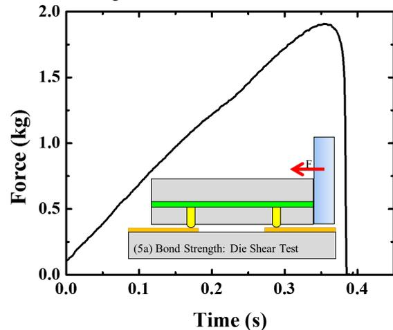
Figure 10: Die shear strength measurement setup (*inset*) and typical die shear strength measurement, showing failure at  $1.9\text{kg}$  applied shear force.
